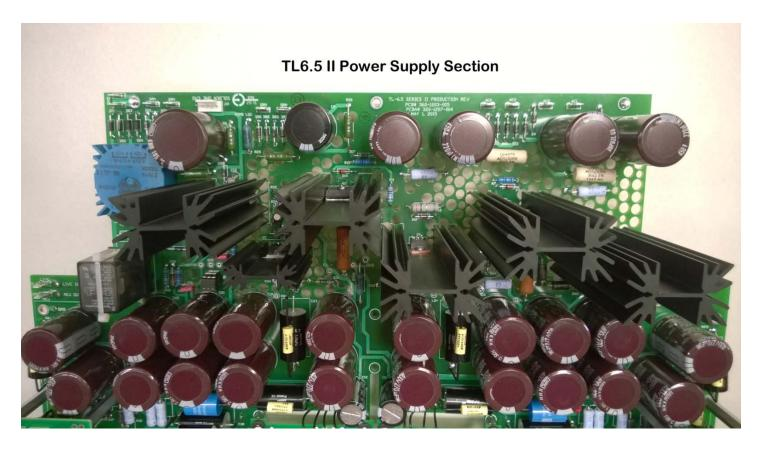
A good solid power supply section with lots of tall heatsinks and ventilation holes.
