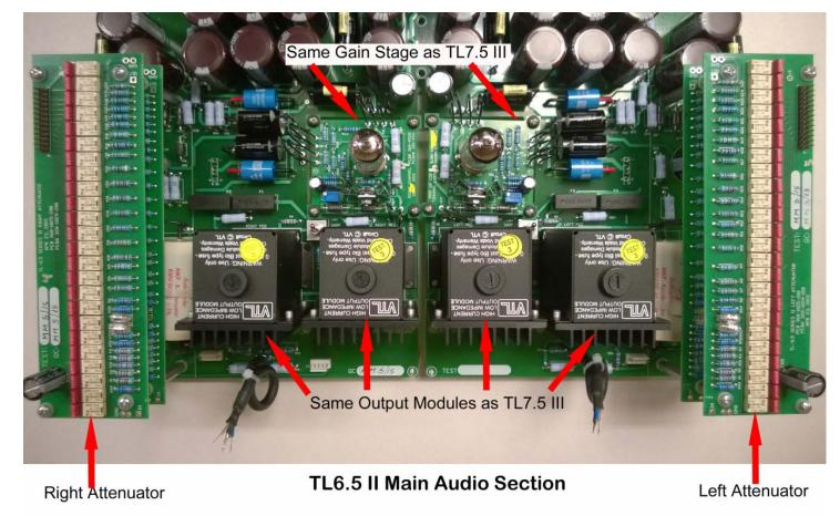
Main Audio section is very similar in layout and configuration as the TL7.5 III. In fact many of the parts are shared between the two models.
